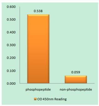
Enzyme-Linked Immunosorbent Assay (Phospho-ELISA) for Immunogen Phosphopeptide (Phospho-left) and Non-Phosphopeptide (Phospho-right), using A-RAF (Phospho-Tyr302) Antibody
